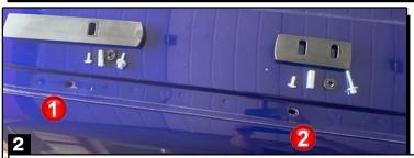
Position 1 has a plastic foot with 1 hole. Whilst position 2 has a foot with 2 holes. Both have a T-bolt, a long hexagonal nut, a large plastic washer with lugs, & a hex-nut (a medium one for position 1 at the rear, and a slightly longer one for 2) In the image shown, we have also fitted the little washer.
