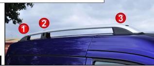
The rails attach to the roof in three places. Positions one and two at the rear of the vehicle are similar, and we will cover these on this page. Position three is slightly more complex and we will cover that over the page.
