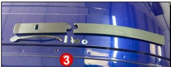
Position three has two unique plastic feet & a bolt with a long plastic holder, the same long hexagagonal nut as before, a medium bolt with a washer, a big flat plastic coated washer, and a big flat metal washer. But notice that the plastic coated washer for position three has no lugs.
