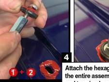
Attach the hexagonal nut, slide the entire assembly into the hole, and turn in place, then tighten with the correct sized spanner.
