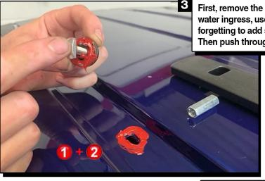
First, remove the blanking covers from the top of the vehicle. Then to prevent water ingress, use the included Red Instant Gasket paste as shown, not forgetting to add some to the large plastic washer and the side with the lugs. Then push through the T-bolt.
